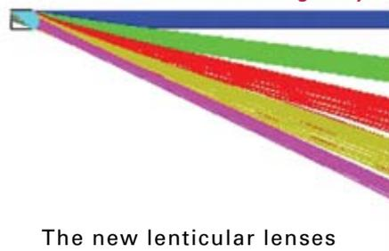
The new lenticular lenses also provides a much wider field-of-viewing angle, as well as brighter, clearer and better contrast images than the typical cylindrical/spherical lenticular lenses.
